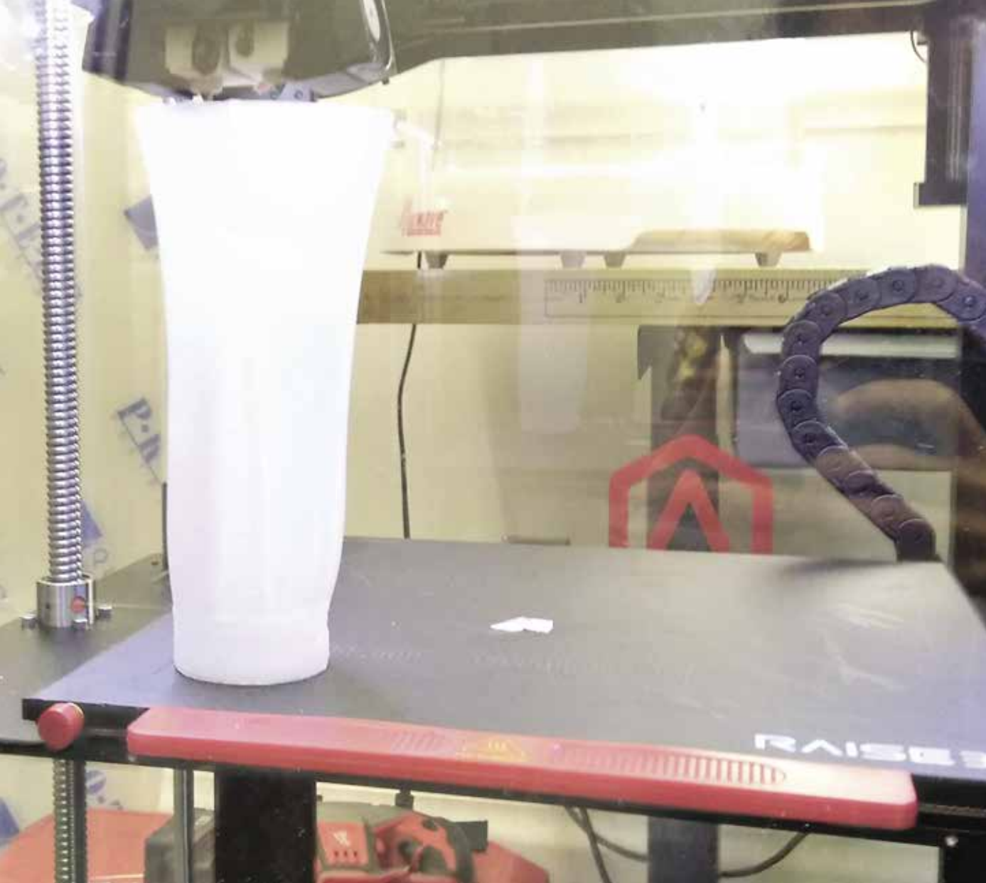
Testing facility, Safa Herfat PhD, Transtibial prosthetic socket being 3D printed for a patient at the OTI O&P clinic (OTI Biomedical Engineering Lab).
